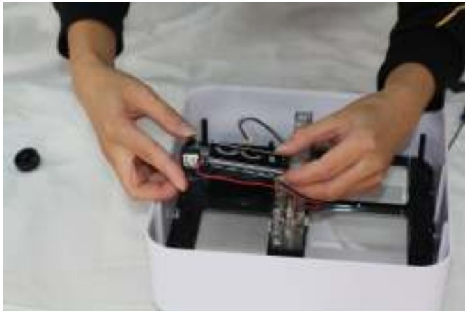
6. Install the Month support board.
