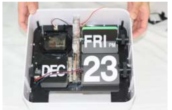
11. Install the Date flips.
