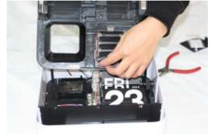
14. Tidy the wires and re-install the battery contact.
