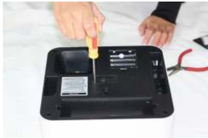
15. Replace the back casing and screw in the 5 screws.
