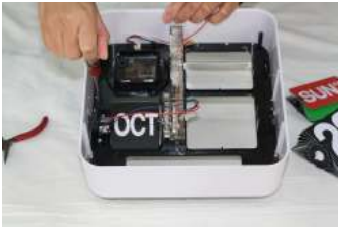
7. Remove the Month support board and 2 screws.
