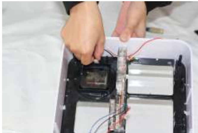
4. Plug in the wire attachment.
