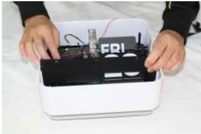
12. Re-install the support board.
