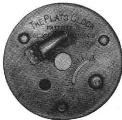
Fig. 17 Movement cover plate for models having detached key. Note special key-holding clamp
