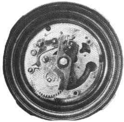
Fig. 24 Movement of Junghans 30-hour model
